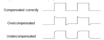
Figure 4.4 Probe compensation4
