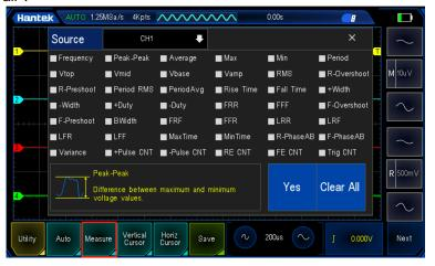
Figure 10.1 Measurement parameters
