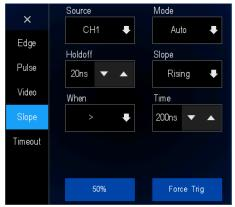
Figure 9.5 Slope trigger menu
