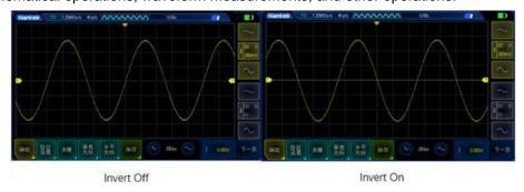
Figure 6.2 Waveform inversion
