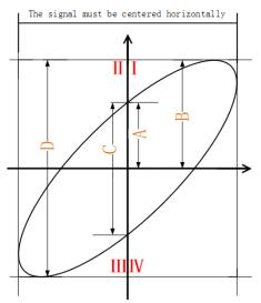
Figure 11.1 Phase difference schematic diagram
