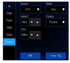
Figure 9.6 Timeout trigger menu
