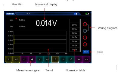
Figure 16.1 Multimeter
