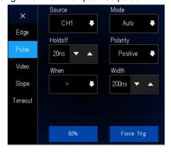
Figure 9.3 Pulse width trigger menu
