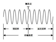
Figure 11.3 Schematic diagram of storage depth
