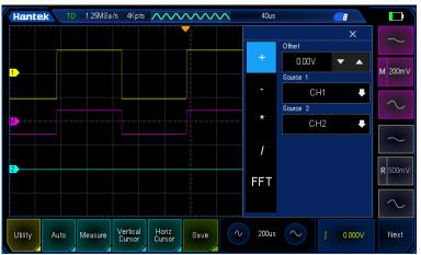
Figure 7.2 Addition operation
